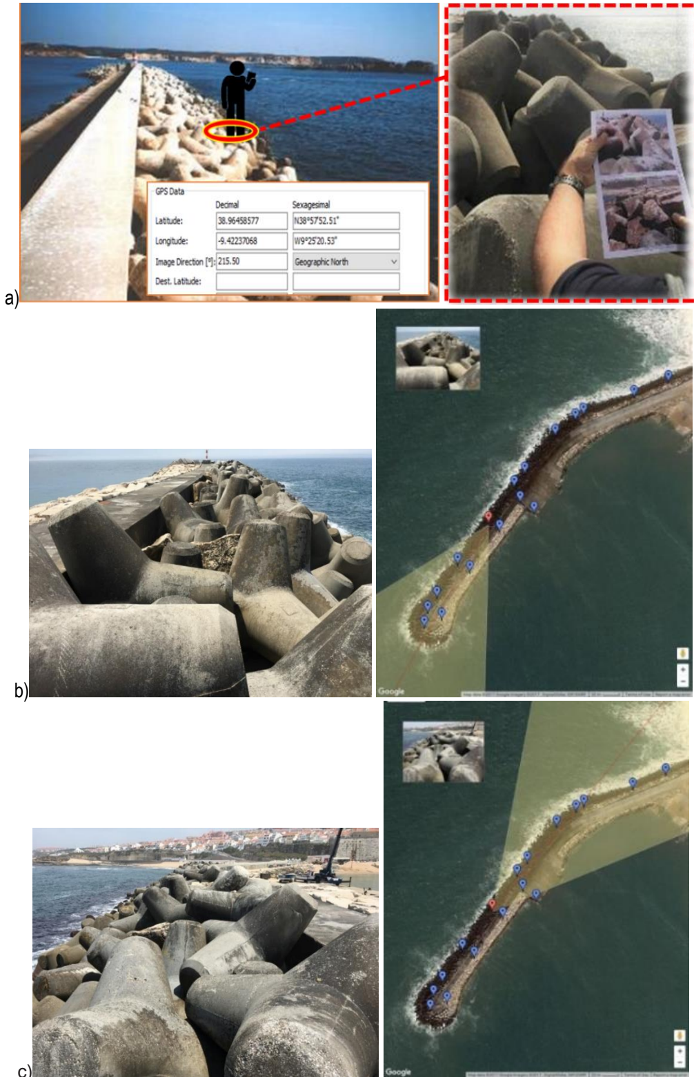
Figure 3 - a) Systematic photographs taken at predefined points. Case of Ericeira's breakwater, according to two predefined directions: b) southwest; c) northeast
