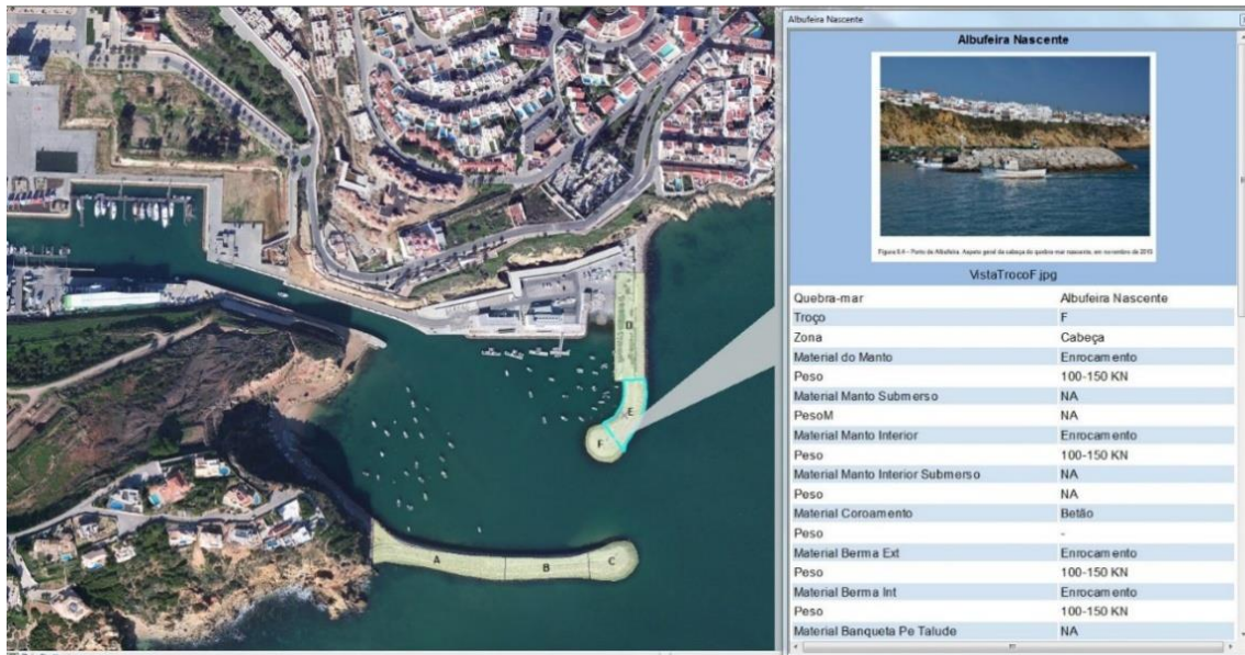
Figure 12 - A search operation in the ANOSOM_GIS interface for construction materials of Albufeira's breakwaters
