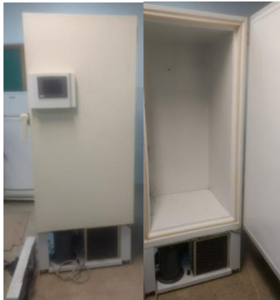
Figure 6 - Freezer front, showing main digital display, and internal chamber.
