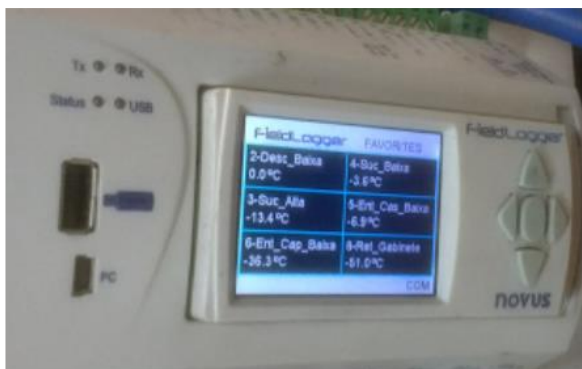
Figure10 - Auxiliary Display, showing real time temperature measurements.
