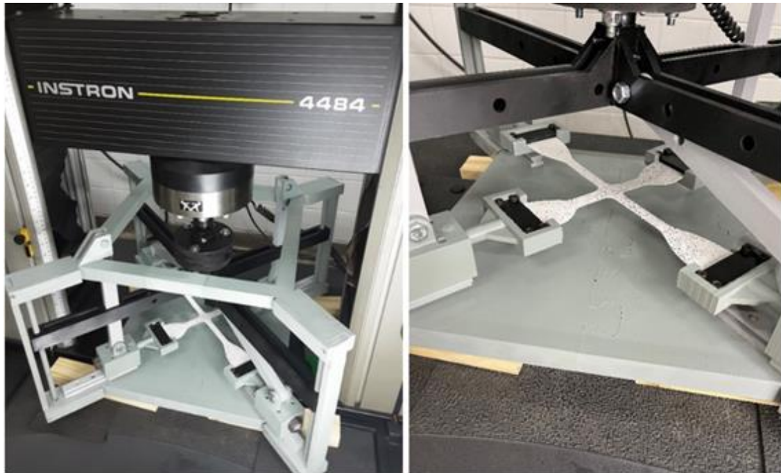
Figure 17: Test setup for in-plane deformation state (1:0).
